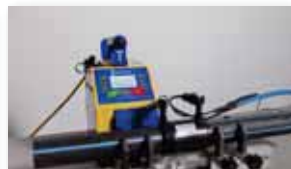
Read the bar code and start welding. Perform the required controls (alignment, depth of insertion and fusion indicators).
