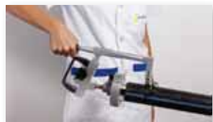
Use the proper scrapers. Clean the surfaces with a suitable detergent.
