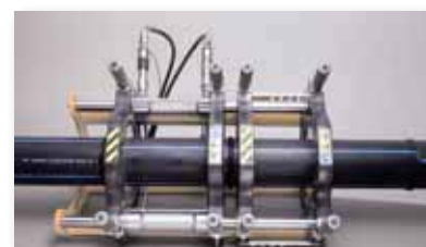
Stage 5 welding with element in pressure
