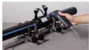
Read the bar code and start welding. Perform the required controls (alignment, depth of insertion and fusion indicators).
