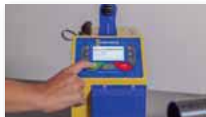
Read the bar code and start welding. Perform the required controls (alignment, depth of insertion and fusion indicators).
