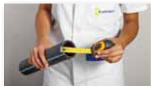
Check the size of the parts to be welded.
